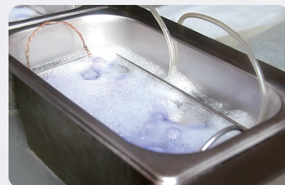
06 Dissolve the support wax in the wax washing solution
