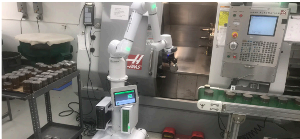
LATHE BLANKS DELIVERED BY CONVEYOR BELT
