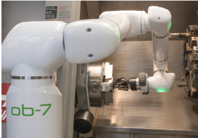
OB7 INSERTS PART INTO A LATHE CHUCK
